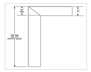
A slightly irregular bowed wall can be accepted as Hartson-Kennedy countertops have a 3/8" scribe which can be sanded or planed to fit bowed walls.
