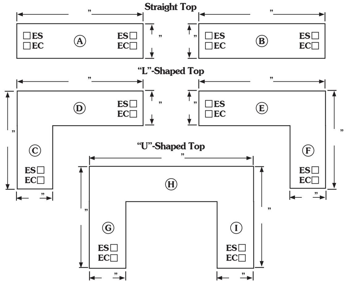
Detail each End Cap (EC) or End Splash (ES) by checking the box provided at every end. Indicate arc ends with dotted lines.
